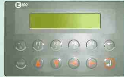
HMI Control Unit
