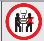
**BEFORE OPERATING THE PRESS AND DURING ITS NORMAL WORK, THE OPERATOR MUST ALWAYS CHECK THAT NO PEOPLE (OR ANIMALS) ARE NEAR THE MACHINE!**
