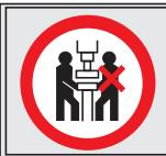
**BEFORE OPERATING THE PRESS AND DURING ITS NORMAL WORK, THE OPERATOR MUST ALWAYS CHECK THAT NO PEOPLE (OR ANIMALS) ARE NEAR THE MACHINE!**
